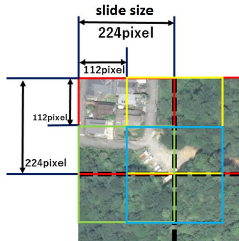
Figure 3: The simple segmentation method and the sliding segmentation method
