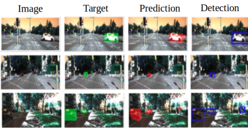
Fig. 3. Segmentation and detection of the "Car" class with Camera.
