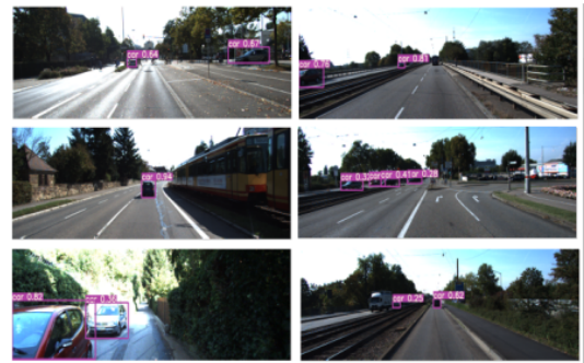
Fig. 5. Detection of the "Car" class with Camera.
