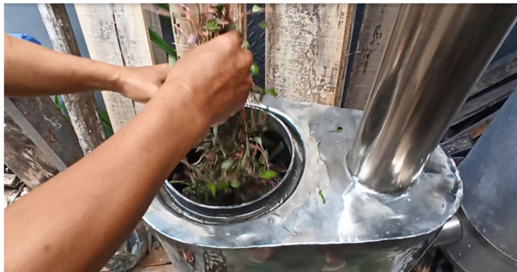
Fig 11. Put the waste into the reactor
