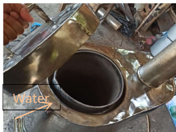
Fig 4. Water as an insulator on reactor
