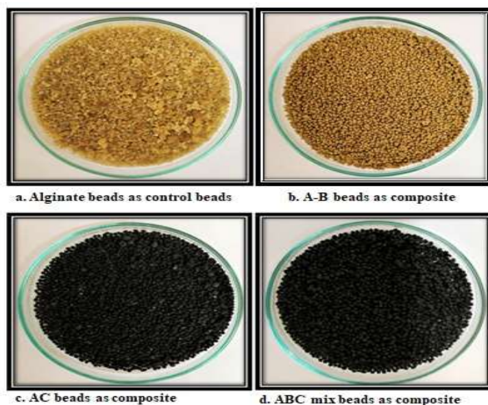
Fig 1. a. Alginate beads as control beads; b. A-B beads as composite; c. AC beads as composite; d. ABC mix beads as composite
