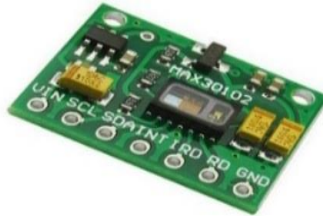
Fig. 5 Pulse sensor with 3 Pin and pulse oximeter Max30102 integrated with PCB circuit
