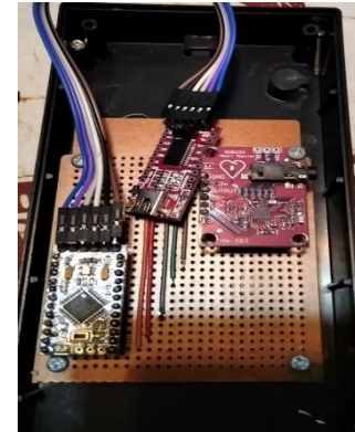
Fig 3. ECG sensor device with PCB circuit
