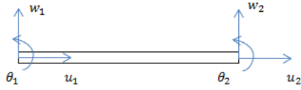
Figure 5. Passive beam element
