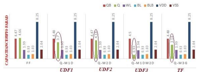
Fig.6 .Fault Detection Based on Parasitic capacitance variation at node Q
