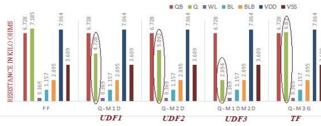
Fig.7. Fault Detection Based on Parasitic Resistance variation at node Q
