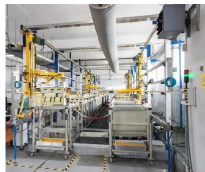
Fig. 1. Immersion electrolytic coating line.
