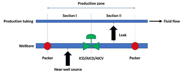
**Figure 7.** Simplified model of a single production zone in the OLGA simulator (Moradi and Moldestad, 2021).
