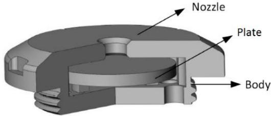
**Figure 2.** Schematic sketch of RCP-type AICDs (Mathiesen et al, 2011).
