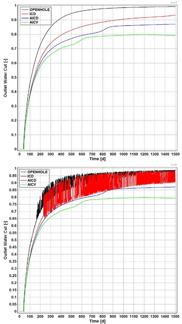
**Figure 12.** Outlet water cut in Case a (up), and Case b (down).
