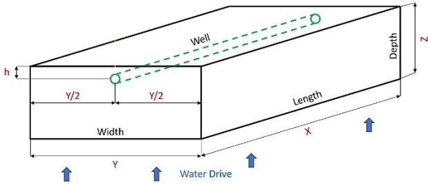
**Figure 5.** Schematic geometry of the reservoir near the well (Moradi and Moldestad, 2020).
