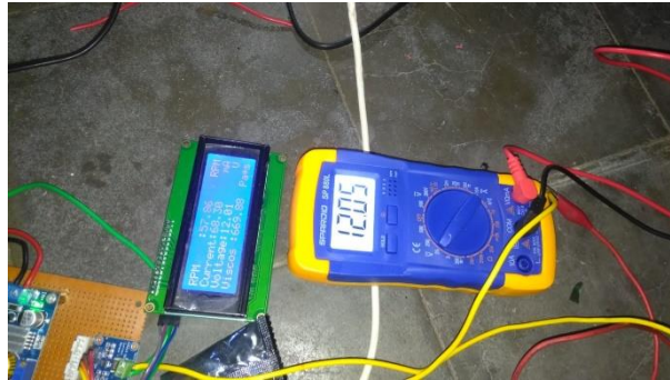
Figure 11. DC motor voltage test
