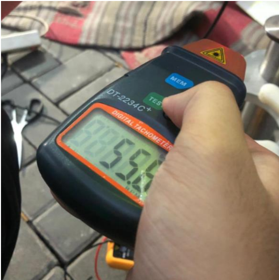
Figure 15. Testing dc motor rpm with tachometer
