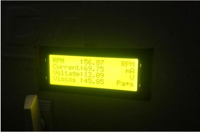
Figure 14. Speed sensor test (optocoupler fc 03)
