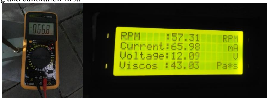
Figure 10. DC motor current test
