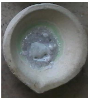
Fig. 5. Photograph of NbP 3 O 10 phosphates inside the alumina crucible at 400°C
