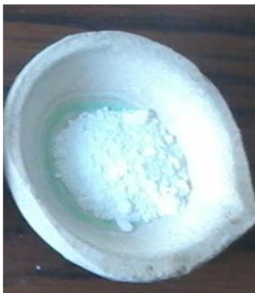
Fig. 4. Photograph of NbP 3 O 10 phosphates inside the alumina crucible at room temperature (25°C)
