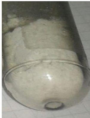
Fig. 7. Photograph of NbP 3 O 10 phosphates inside the alumina crucible at 1000°C after grinding
