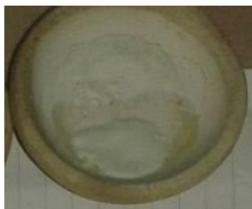
Fig. 6. Photograph of NbP 3 O 10 phosphates inside the alumina crucible at 1000°C before grinding
