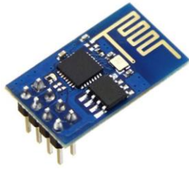
fig.5: ESP8266 with on-board Wi-Fi antenna
