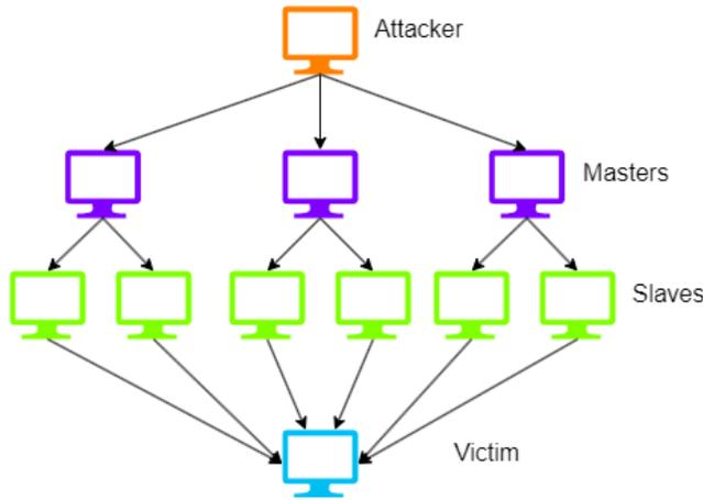
Fig. 2. DDoS attack architecture diagram
