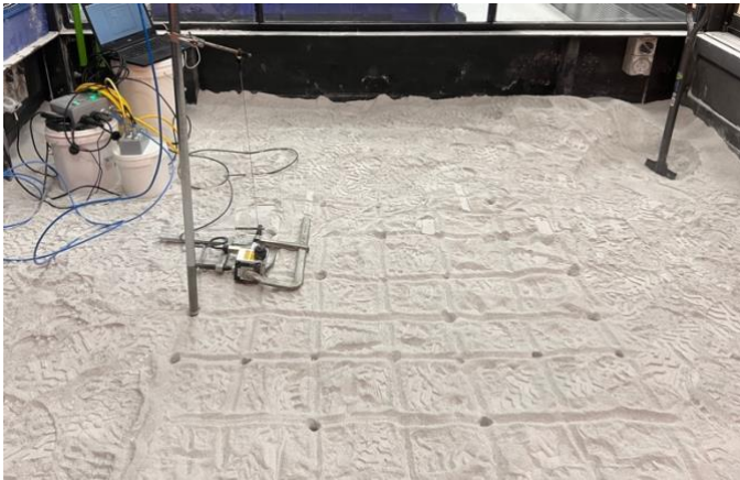
Fig. 3. Cone penetration resistance measurements in the Regolith pit at EXTERRES lab.
