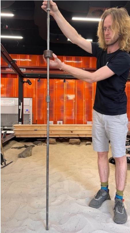
Fig. 1. Mini dynamic cone penetrometer (Mini-DCP) demonstration in the sand pit, EXTERRES lab, University of Adelaide.
