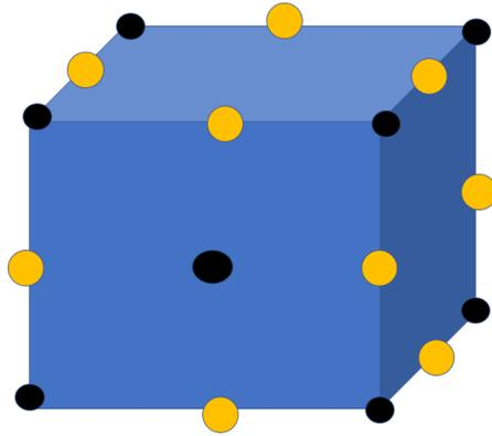
The unit cell of CaTiO<sub>3</sub> is seen as an example of the perovskite structure shown above in this diagram. The presence of Ca<sup>2+</sup> is shown by black holes at the cube's corners. The yellow holes in between the two Ca<sup>2+</sup> ions represent O<sup>2-</sup>.
