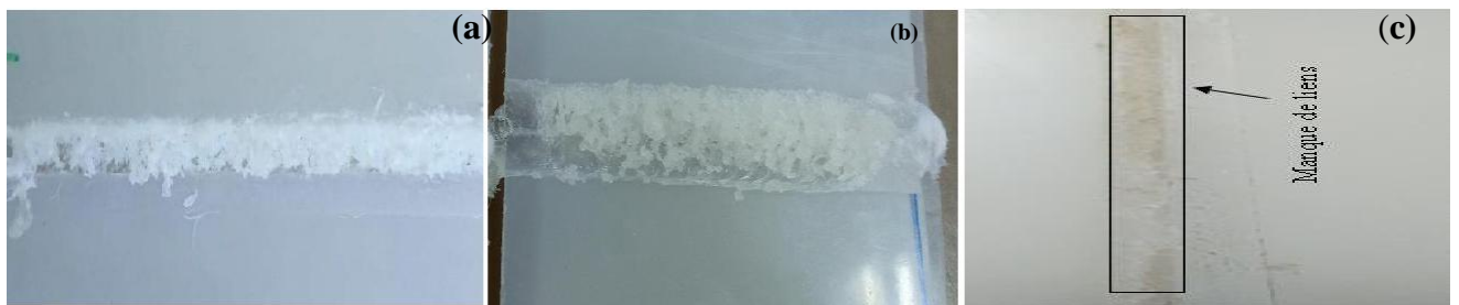
Figure 6: Welding states, (a): rotation speed less than 500 rpm, (b): rotation speed more than 1000 rpm, (c):welding speed 12 mm/min
