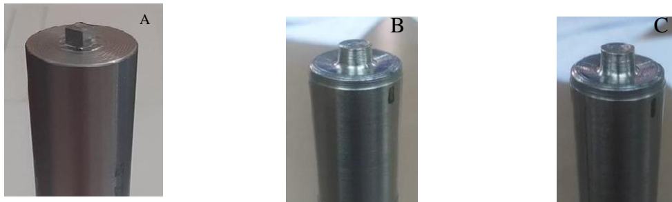
Figure 2: Welding tool: A: square pawn with flat shoulder, B: conical pawn with flat shoulder C: conical pawn with concave shoulder
