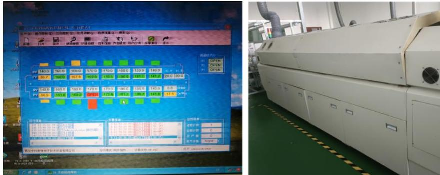
Figure 5. Reflow oven each temperature zone setting and reflow oven
