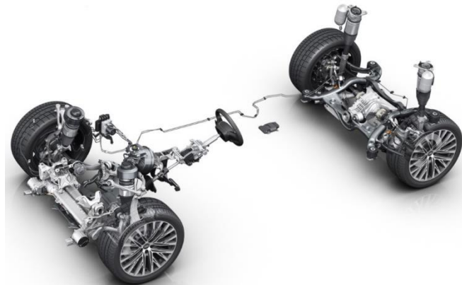
Fig. 3. Electronically driven 4WS steering system [6]
